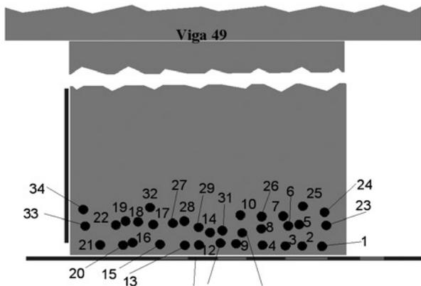
Figure 5. Tomographic results for the case of a 27" thick beam with 34 rebars
