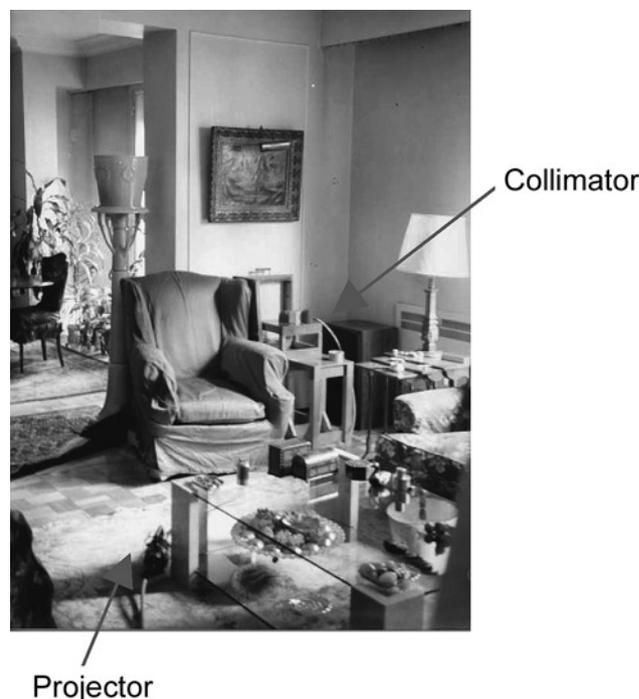
**Figure 4. Example of 'field work' in an inhabited apartment showing how little disturbance is produced by RCT. The lower arrow points to the projector on the floor next to the coffee table. The upper arrow indicates the collimator housing the source during irradiation. This study uncovered the honeycombing defect shown in Figure 2**
