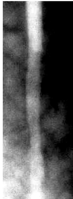
**Figure 3. Portion of a gammagraphy showing corrosion in a rebar, obtained with an Ir192 source**
