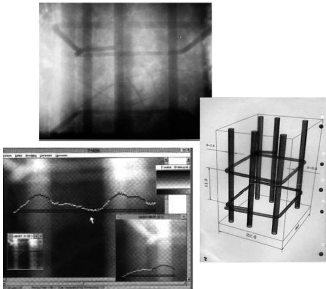
**Figure 1. Gammagraphy of a column with six 16 mm  $\phi$  rebars and stirrups obtained with a Cs137 source; digitised portion of it and 3D reconstruction**
