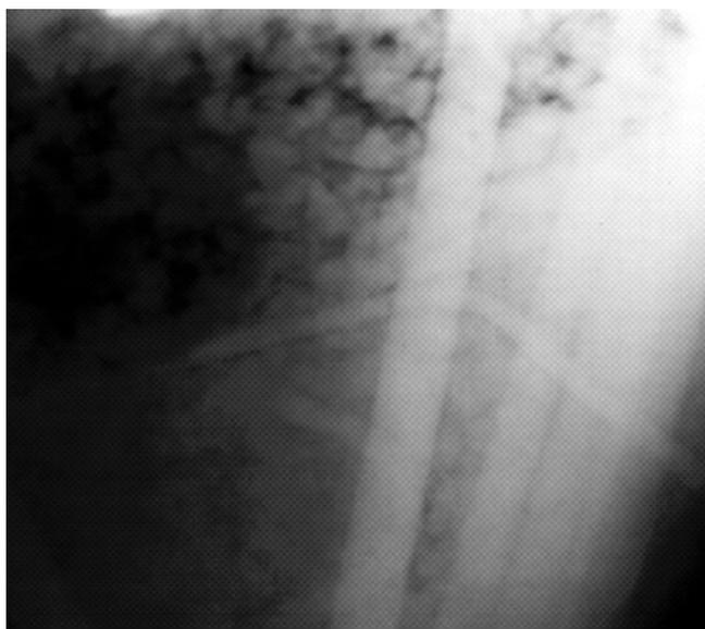
**Figure 2. Evidence of honeycombing in an inclined column (corresponding to study shown in Figure 4). Obtained with an Ir192 source**
