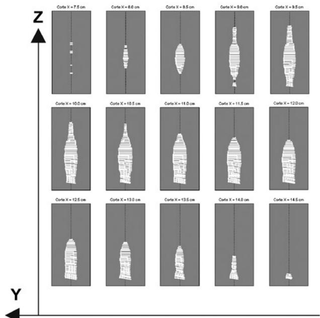
**Figure 8. Air length equivalent in the plane parallel to radiation, for different values of the coordinate perpendicular to radiation. Unlike gammagraphy, a single scan provides a measure of the amount of air along each gamma ray path. In the case shown here it has been assumed that the amount of air along each gamma ray path is uniformly distributed around the centre of the block**
